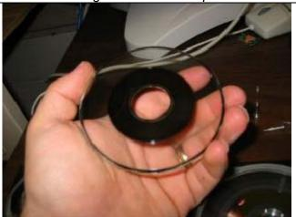
After popping out the first platter I realized that I was correct. The drive platter was now see through. It appears that the head crash scrubbed the drive so clean that the magnetic substrate has been wiped clean off the platters.
