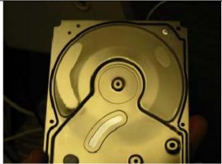
The lid came right off. The first thing we noticed was that there was a large amount of magnetic dust stuck on the lid of the drive. I wiped my finger in one place just to verify that this was not a part of the original manufacture process.
