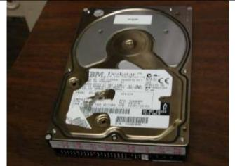
The first step was to remove the screws on the drive lid. I suspect this voided the warranty, but we were on a mission.
